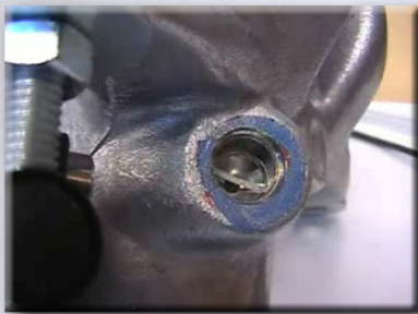
Fine chips residual in the bolt hole and...
